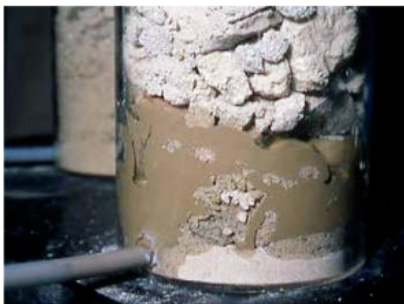
Figure 3.7 Injection of the cylinder in laboratory, (Source: POLIMI).
