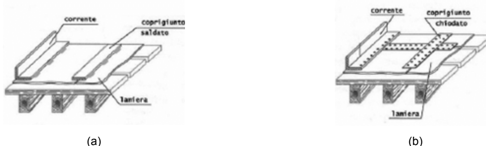
Figure 6.7 In-plane stiffening of floors with metallic plates: (a) welded plates, (b) nailed plates, (Giuriani and Plizzari, 2003).
