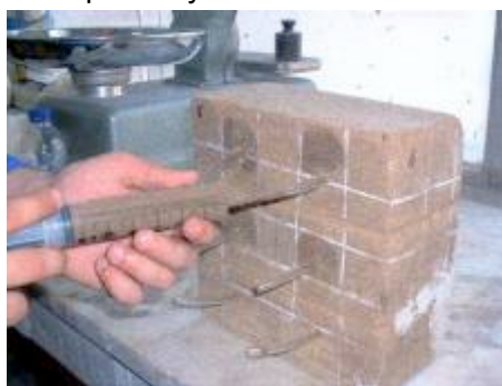
Figure 3.56 Alternative method for repair/strengthening of clay masonry, (by courtesy of Papayianni, 2006).
