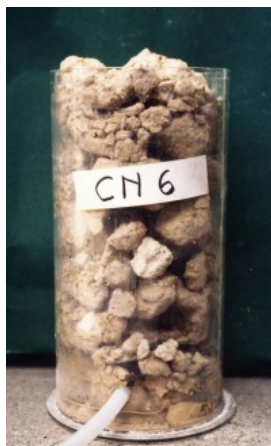
Figure 3.6 The transparent cylinders filled on site by internal leaf materials, (Laefer et al., 1996) and (Binda et al. 2003b,c).
