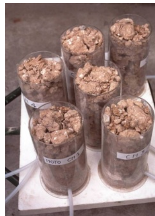
Figure 3.6 The transparent cylinders filled on site by internal leaf materials, (Laefer et al., 1996) and (Binda et al. 2003b,c).
