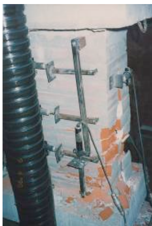
Figure 3.17 Spalling of bricks due to incomplete filling of mortar joints during deep repointing.
