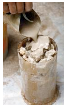
Figure 3.6 The transparent cylinders filled on site by internal leaf materials, (Laefer et al., 1996) and (Binda et al. 2003b,c).
