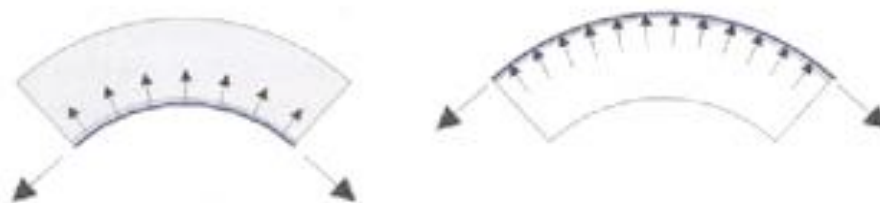
Figure 5.4 Behaviour of FRP at intrados or extrados, (Gurrieri, 1999).
