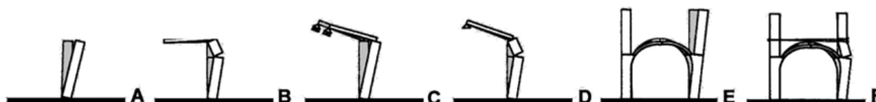
Figure 4.1 Effects of the constraints imposed by floors and vaults, (Carocci, 2004). A unconstrained wall, B floor constraint; C wall not restrained by roof structures; D roof restraining; E vault thrusting; F tied vault.
