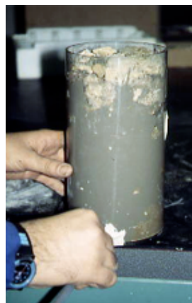
Figure 3.7 Injection of the cylinder in laboratory, (Source: POLIMI).
