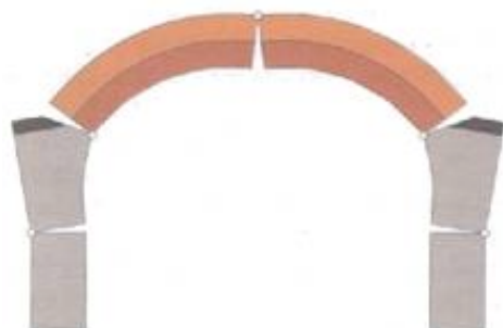
Figure 5.2 Reinforcement arch at intrados, (Gurrieri, 1999).
