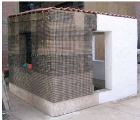
Figure 3.48 Adobe test-house reinforced with polymer mesh and partially plastered.
