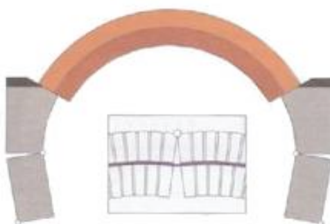
Figure 5.3 Reinforcement arch and FRP, (Gurrieri, 1999).
